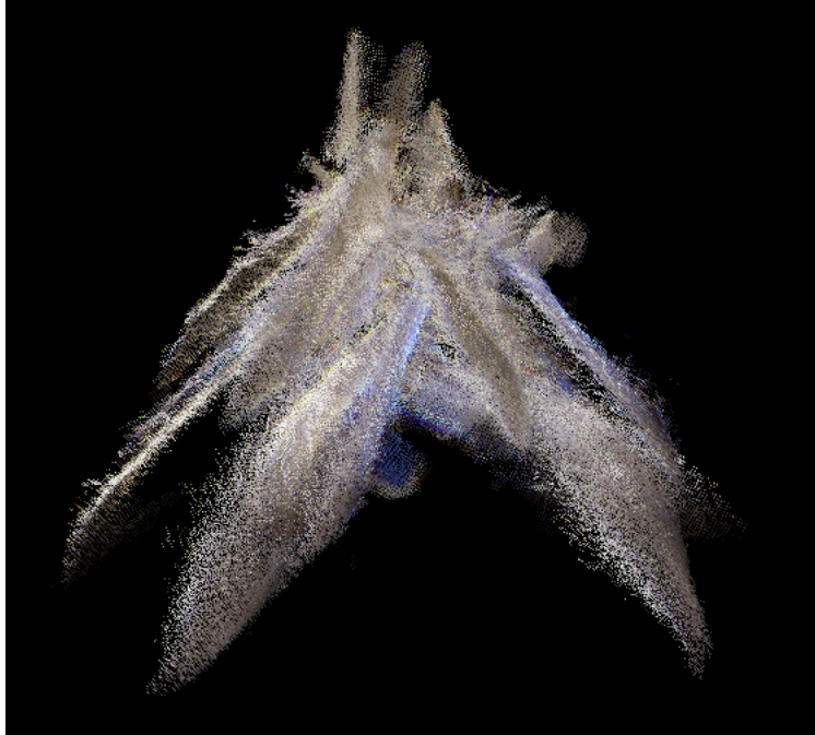
Figure 2.13: Incorrect frame alignment caused by combining successive homogeneous transforms from ICP
